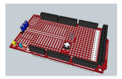
The kit includes the board and many extra components. What you finally end up installing on the ProtoShield will be based on your requirements. But in general, I recommend soldering all the female headers, as they are needed to bring all the signals and POWER from the chipKIT Max32 board to the ProtoShield.
